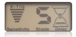
Easy view internal LCD screen showing currently set ADF settings - "X-TIG" function, shade level and delay setting
